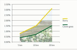
If you want to keep the  $CO_2$  loss below 1 per cent, the average distance should not exceed 7.5 km. This means that suppliers' distance to the biogas plant must be within a radius of 15 km - or that biogas plants must be max. 30 km apart.
